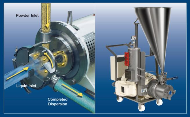
An intense vacuum draws powders including silica, thickeners and pigments into the mix chamber of the SLIM Solids/Liquid Injection Manifold. They are injected through a ported rotor directly into the high shear zone and dispersed instantly. SLIM eliminates the clogging and poor dispersion quality associated with eductor-based systems. It also eliminates the need for an auxiliary pump in most applications. Operation is simple – and the portable inline SLIM easily serves multiple process lines.
