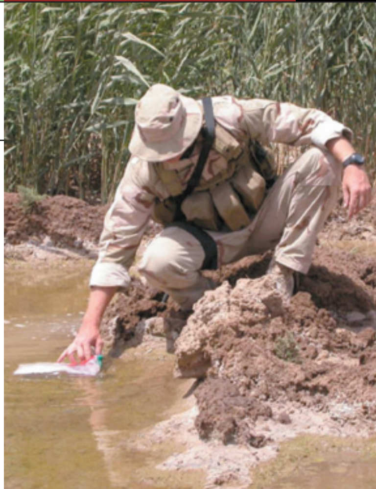
Figure 1. A soldier puts an HTI X-Pack filter into a puddle. The membrane bag will fill with clean water via forward osmosis.
