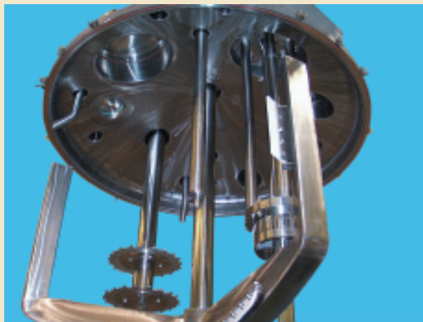
Figure 4. This unit combines a three-wing anchor with scraper, a two-blade, high-speed disperser, and a rotor/stator high-shear mixer. It also features a dished cover with angled ports for adding solvent.
