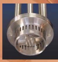
The **Slotted Head** provides the most popular combination of high shear and efficient flow rates. It is well-suited for emulsions and many medium-viscosity mixing applications.
