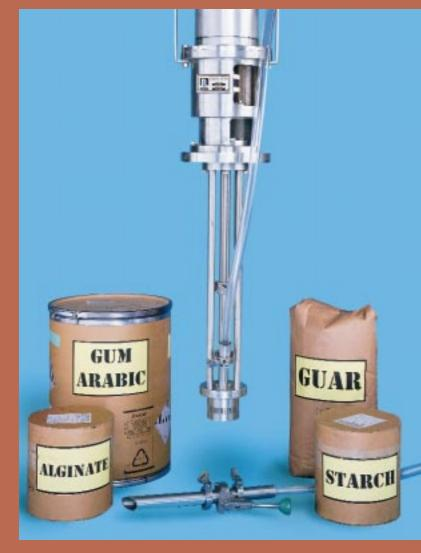
**Model 505 Stainless Steel High Shear Mixer with batch SLIM system: 5HP** – While the mixer is running, the operator simply inserts the feed tube into a container of powder and opens the feed valve. The vacuum created by the specially modified rotor/stator generator draws the powder through the tube and directly into the high shear zone. Dusting and delays are eliminated.
