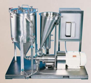
**Model 405SB-25: 25 HP** – This skid-mounted system includes an In-Line SLIM and a 50-gallon jacketed recirculation vessel for high-speed powder induction. Skid-mounted systems can be wheeled from one vessel to another to accommodate a variety of process lines. Ross can provide a custom-designed skid-mounted system, including the mixer, vessel, piping and valves, pump and complete controls, to meet the demands of any application.
