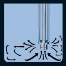
The rotor/stator generator of the batch High Shear Mixer is generally positioned 2-3 head diameters from the bottom of the vessel, and slightly off-center. To ensure adequate suspension of heavier solids, the rotor/stator generator may be located in the center of the vessel.
