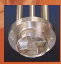
The **Fine Screen Head** applies the highest shear rates of all single-stage High Shear Mixers. It is generally used for lowerviscosity emulsions and fine dispersions.
