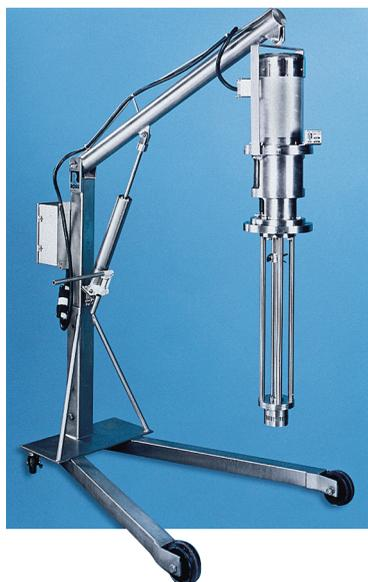
Portable High Shear Mixers like this one can be moved easily from one vessel to numerous other vessels. With proper positioning of the rotor/stator generator within the vessel, these mixers can efficiently handle batch sizes up to about 1,000 gallons.
